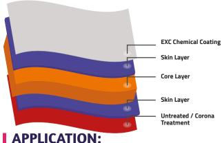
• Film is designed for direct extruded Polyethylene adhesion without the need for primer
